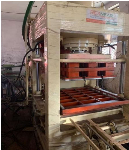
Hydraulic brick Press machine
