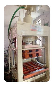
Non-Fired Good Bricks = Soil (90%) + Cement (9.8%) + Soil Stabilizer (0.2%)
